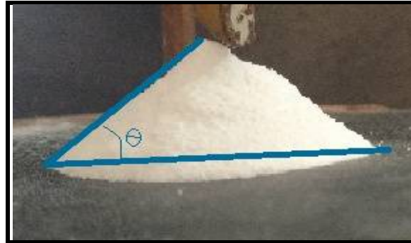
Fig. 1 Angle of repose measurement of pile of iodized salt
