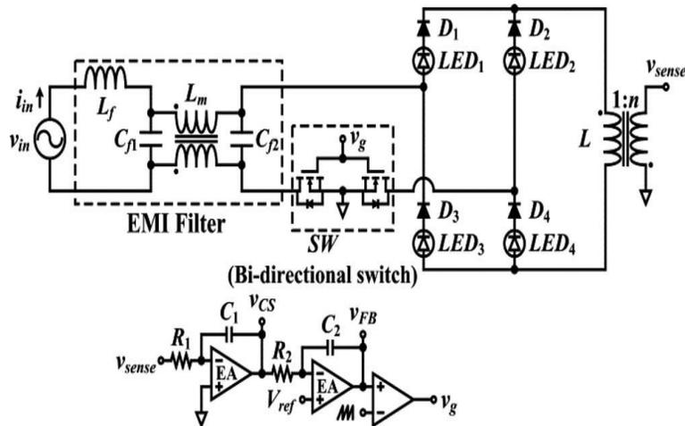
Fig.2 Circuit Diagram
