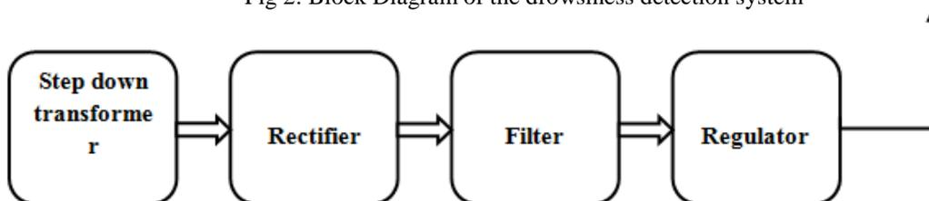
Fig 3: Regulated power supply
