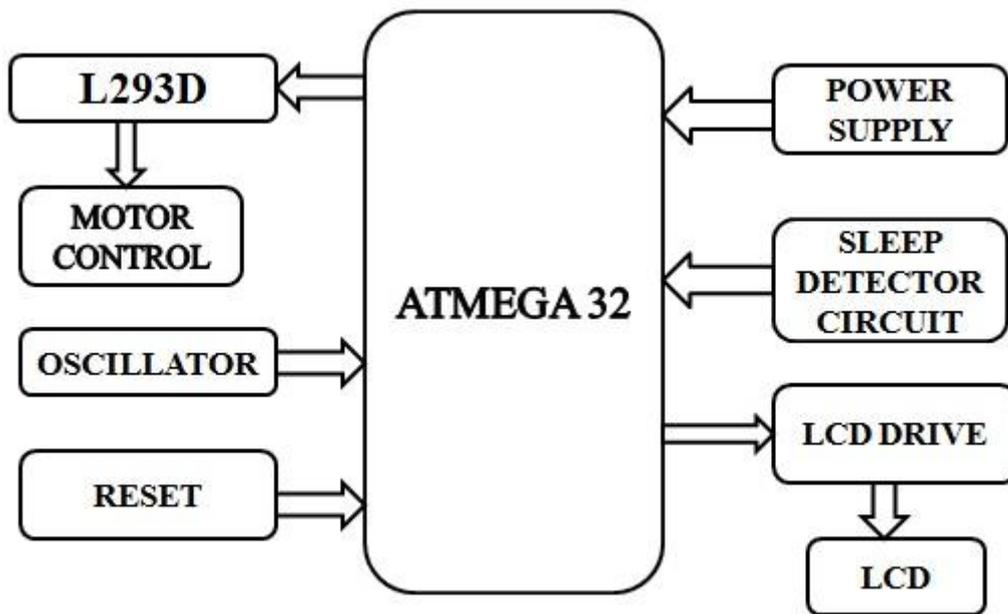
Fig 2: Block Diagram of the drowsiness detection system
