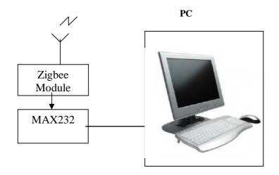
Fig 2.Receiver Section of the Wireless Monitoring System
