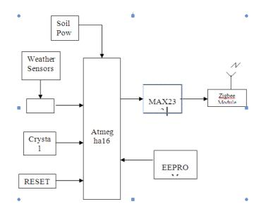
Fig 1.Transmitter Section of the Wireless Monitoring System
