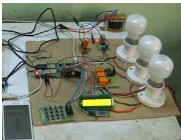
Fig.7 Shows test set up of Raspberry pi based Central office room
