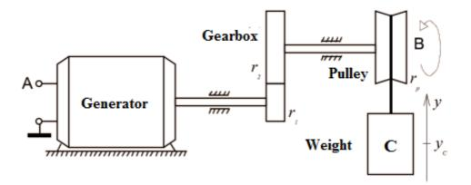
Fig. 2 Experimental setup of energy generated from weight lifting technique with gearbox
