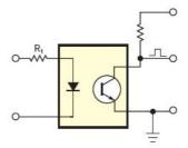
Fig 3: Optocoupler structure
