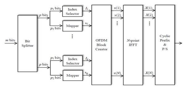
Fig 1: OFDM-IM Block Diagram
