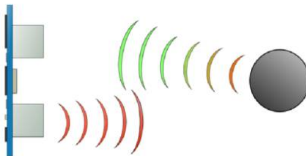
Figure 6. Functioning of an ultrasonic sensor
