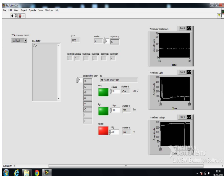
Figure 4.4 Testing results when Voltage exceeds
