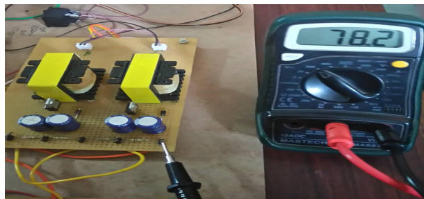
Figure 10. Voltage across each capacitor
