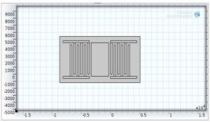
Fig. 5. Design of SAW Device
