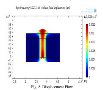
3. SAW Device – Design 3: In the Design 1 of SAW Device, the metal (Aluminium) is used in interdigitated transducer and the sensing layer is made up of Lithium Niobate between the two IDT's. The piezoelectric material used as the substrate. Here the finger spacing is up to 600µm. By applying the value of the Eigen frequency, the corresponding displacement and potential are tends to be measured which is shown in "Fig. 10" and "Fig. 11".
