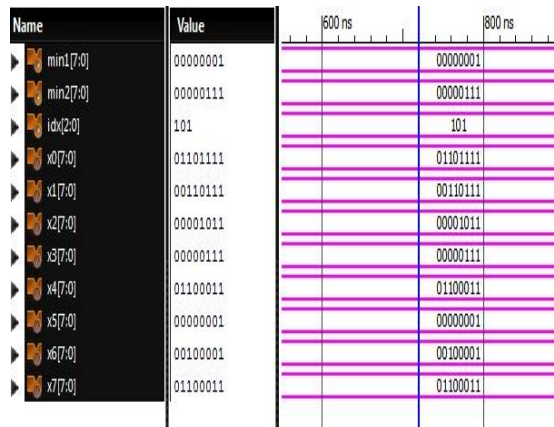
Fig:9. Simulations results of 8-bit Proposed searching module.
