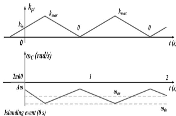
Fig. 7. First PLL output behavior when the islanding condition occurs.
