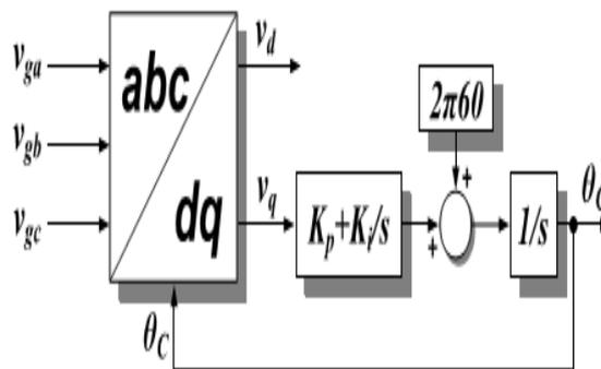
Fig. 1. Synchronous reference frame PLL linear model.
