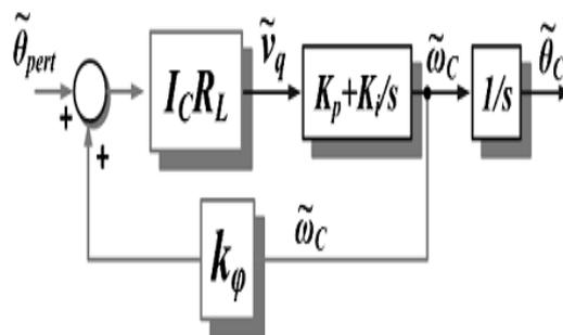
Fig. 5. Linearized small-signal PLL model under islanded condition.
