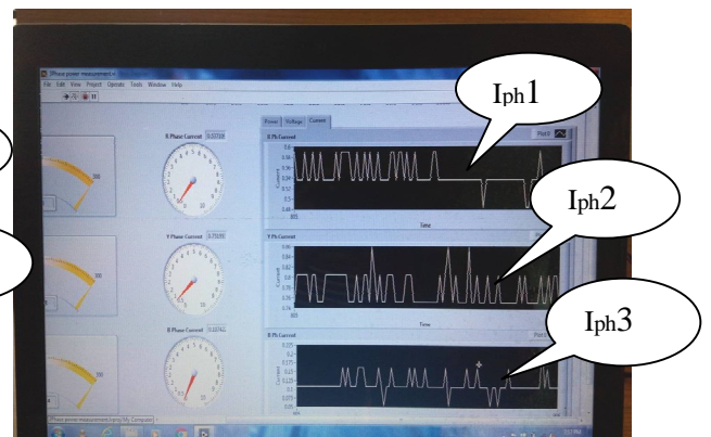
Fig 11: Current Waveform Obtained in LAB View with controls and indicators
