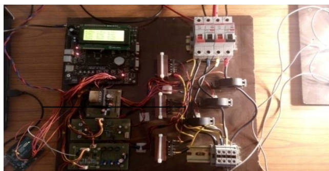
Fig 3 Hardware setup for data acquisition by Connecting Lamp as a Load
