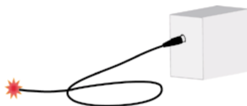
Figure 5: Phosphor Sensor at the End of the Fiber Optic Probe excited by an LED in the Instrument
