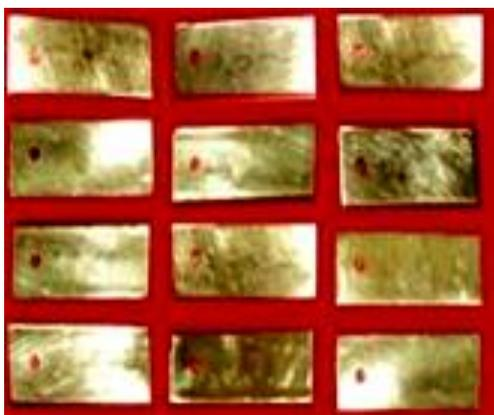
Fig. 5 Slurry Eroded Test Specimens of Uncoated Naval Brass
