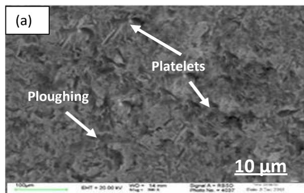
**Fig. 10 (a) SEM Image of Uncoated Naval Brass at Higher Impact Angle(90<sup>0</sup>)**
