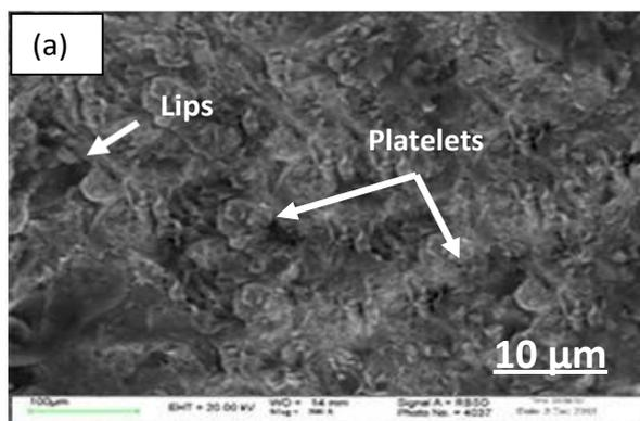
**Fig. 9(a) SEM Image of Uncoated Naval Brass at Moderate Impact Angle(60<sup>0</sup>)**
