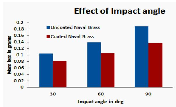
Fig. 7 Effects of Impact Angle on Erosion Rate Of Uncoated and Coated Naval Brass
