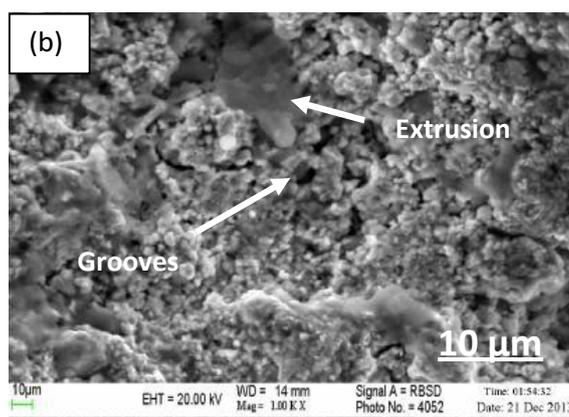
**Fig. 8 (b) SEM Image of Coated Naval Brass at lower impact angle(30<sup>0</sup>)**
