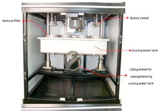
Fig.1 Slurry Erosion Test Setup
