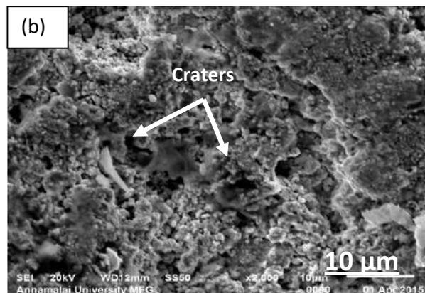
**Fig. 10 (b) SEM Image of Coated Naval Brass at Higher Impact Angle(90<sup>0</sup>)**
