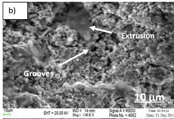
**Fig. 9(b) SEM Image of Coated Naval Brass at Moderate Impact Angle(60<sup>0</sup>)**
