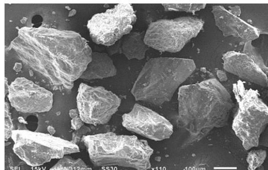
Fig. 2 SEM image of Quartz sand
