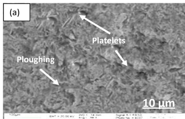
Fig.8(a) SEM Image of Uncoated Naval Brass at Lower Impact Angle(30°)
