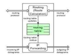
Fig 2. Functions of a router.
