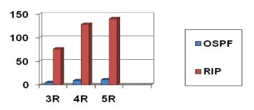
Fig 8. Graph of the comparison of packet loss with 3, 4 & 5 routers
