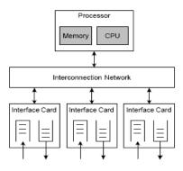
Fig 1. Router components.
