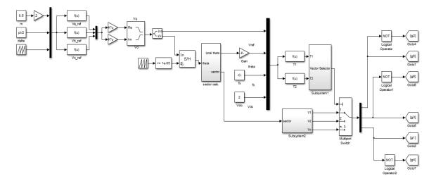
Fig 3: Space Vector PWM Simulink Block.
