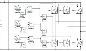
Fig. 2 :2 level voltage source inverter using IGBTs
