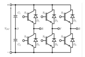
Fig 1: 2 level voltage source inverter using IGBTs
