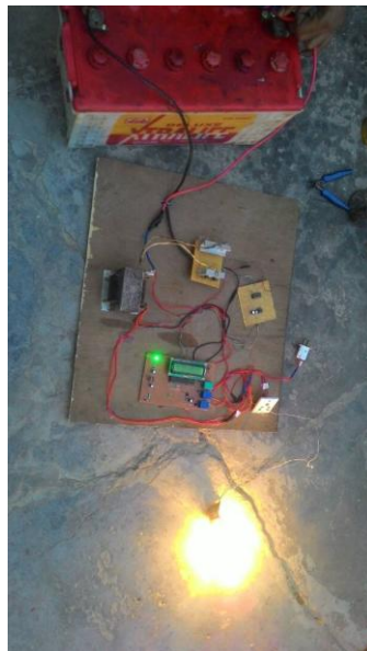
Fig 5 Bulb glowing through output from inverter
