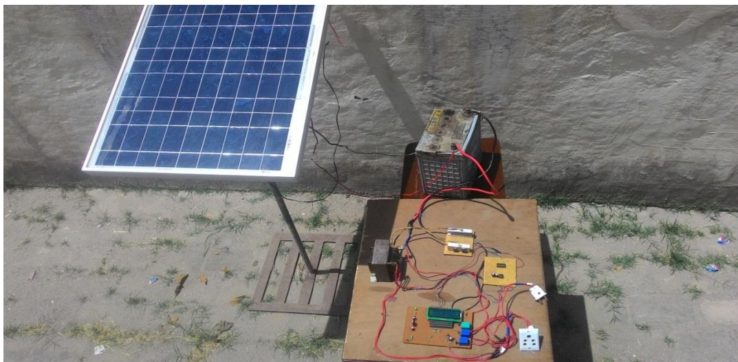
Fig 3 Assembled prototype of solar inverter
