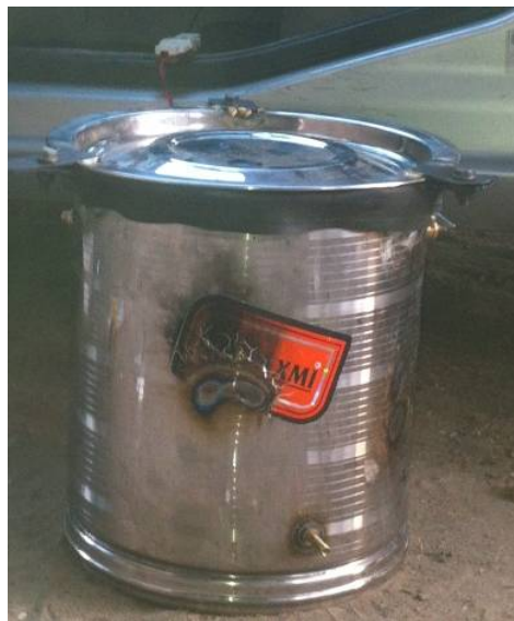
Fig. 3 Portable vacuum system.
