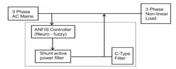
Fig. 1 : Block-diagram of the neuro-fuzzy inference scheme to suppress the harmonic contents in the supply voltage and to improve the power quality
