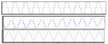
Fig. 7 : Plot of load current before and after the incorporation of the ANFIS (Artificial Neural Network's Neuro-Fuzzy) controller .... before, imbalance seen due to switching, after ANFIS controller, balance seen
