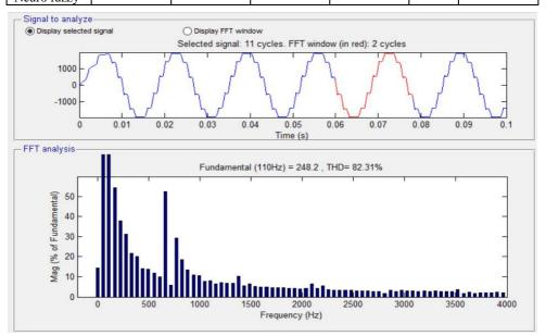
Fig. 8 : Waveform Showing the THD before Applying Compensation Using ANFIS (V)
