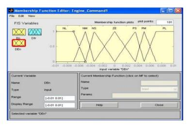
Fig. 3 : Fuzzy membership functions developed in Matlab
