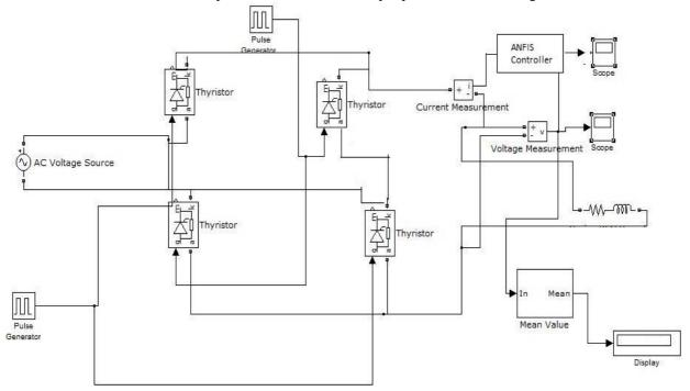
Fig. 4 : Developed simulink model for ANFIS controller for harmonic eliminations
