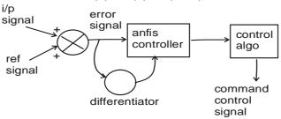
Fig. 2 : Illustration of a typical ANFIS Controller with 2 Inputs
