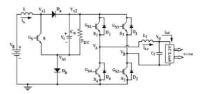
Fig. 1 CFSI topology connected to grid
