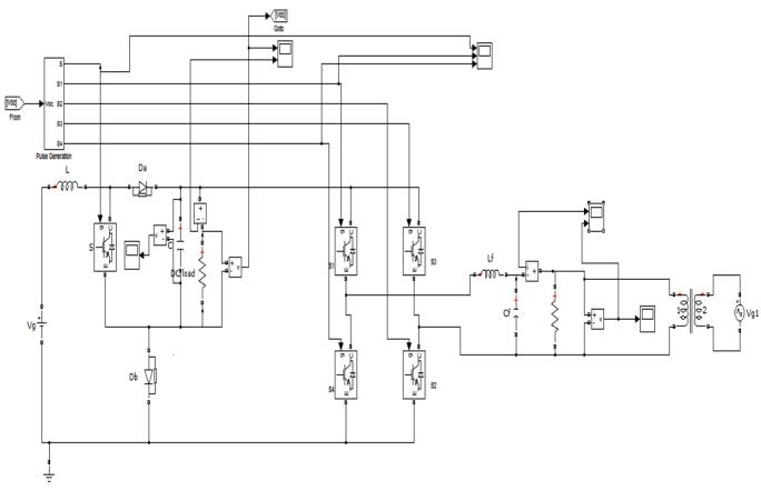
Fig. 4 Simulink model of CFSI based power grid system
