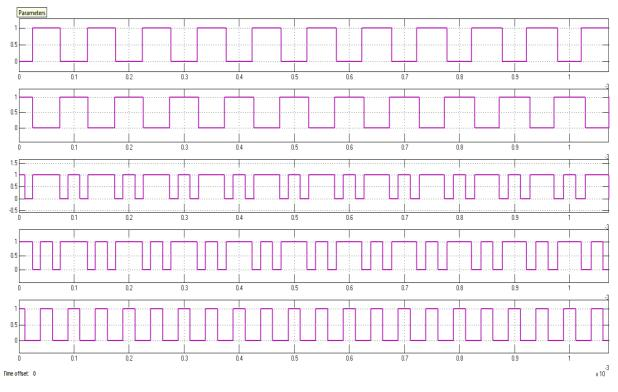
Fig. 5Gating pulses for switches S1, S2, S3, S4 and S respectively
