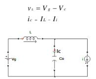
Fig. 3CFSI topology in non shoot-through interval
