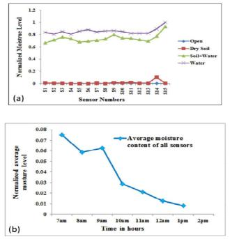
Fig.7 (a) Normalized data of moisture levels vs 15 number of homemade sensors. (b) Average moisture content of all homemade sensors.
