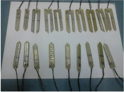
Fig.1 Lab made sensors with different patterns.
