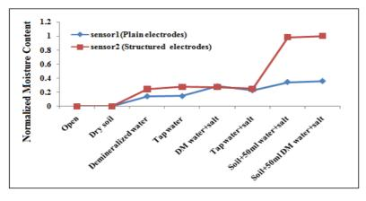
Fig.5: Sensitivity of existed sensors
