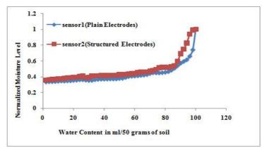
Fig.6: Normalized sensed value corresponding to water content in ml/50grams of soil in a container.
