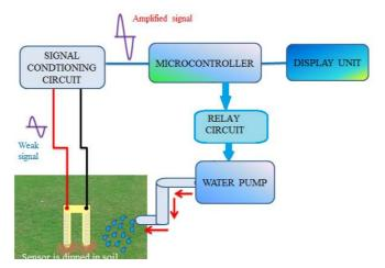
Fig.2.Block diagram irrigation system
