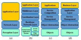
Figure 3 the IoT architecture (a) Three-layer. (b) Middle-ware based. (c) SOA (d) Five-layer.
