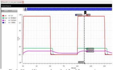
Fig. 8. Vin and Vout waveforms for 1.2 to 0.2v conversion
