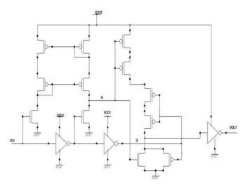
Fig. 2. MWCM based LS using stacking technique.
