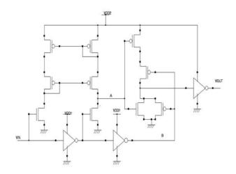
Fig. 1. MWCMHB level shifter.
