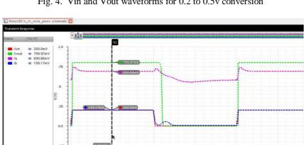
5.0 Fig. 5. Vin and Vout waveforms for 0.2 to 0.8v conversion
