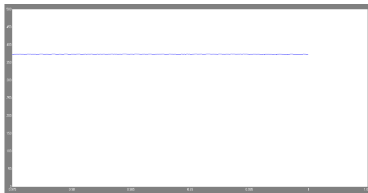
Fig.5 voltage waveform at the high voltage side of high step up single input dual output dc dc boost converter without MPPT
