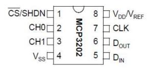
Fig 3: ADC MCP3202
