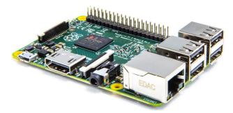
Fig 1: Raspberry pi 2 Model B board
