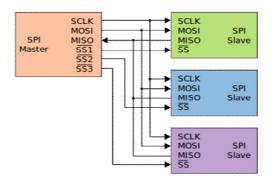
Fig5: 3SPI Slave Devices Connected to Single SPI Master Device.
