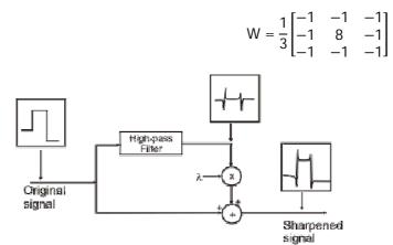
Figure 2:Sharpening Filter
