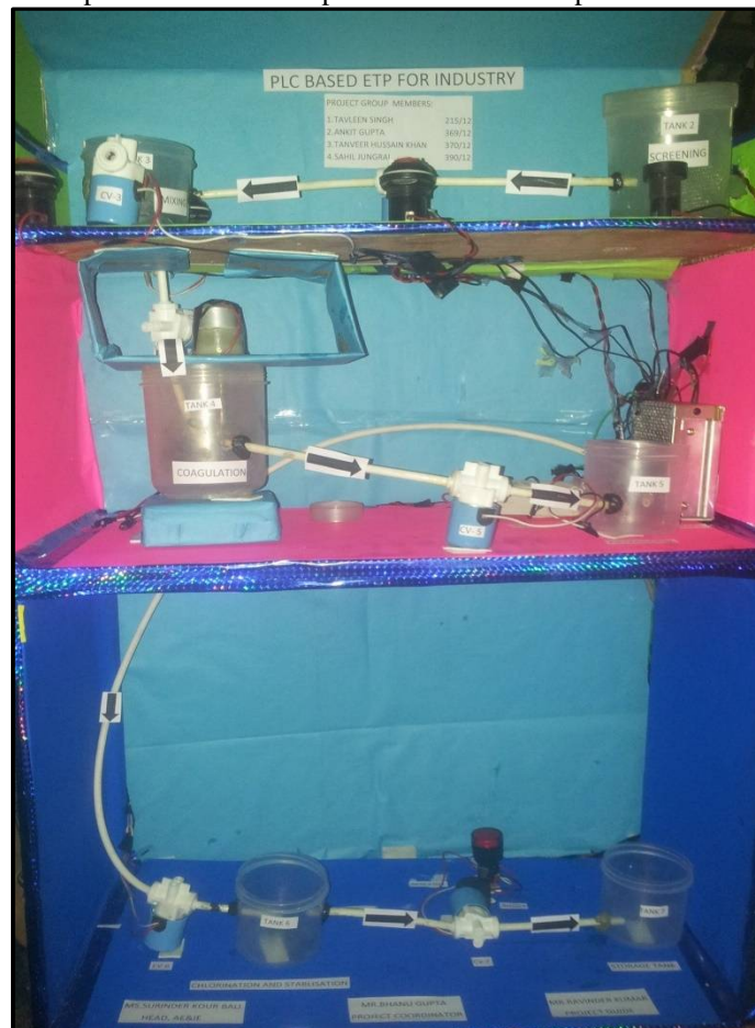
Fig. 8 Hardware Implementation of process control
