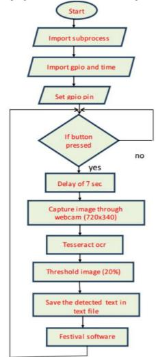
Fig.5 Flow chart of text-to-speech device program
