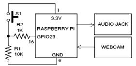
Fig.2 Circuit connection to Raspi board
