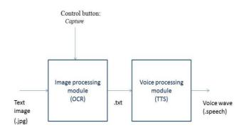
Fig.3 Block Diagram of Text-To-Speech Device
