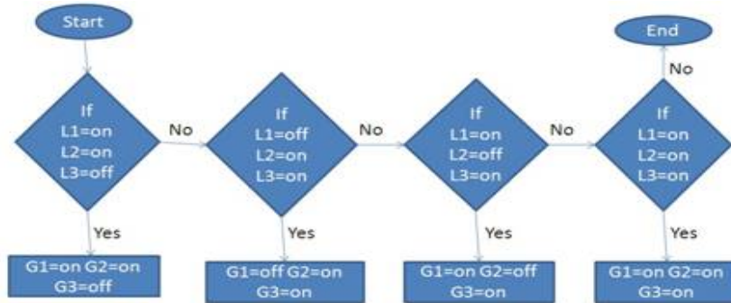
Fig.6 Flow diagram for combination of loads
