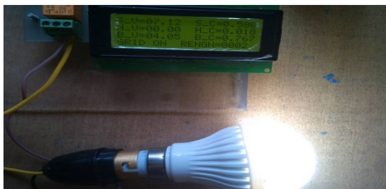
Fig 6: when renewable sources output is too low and battery voltage is low, load connection will be on GRID
