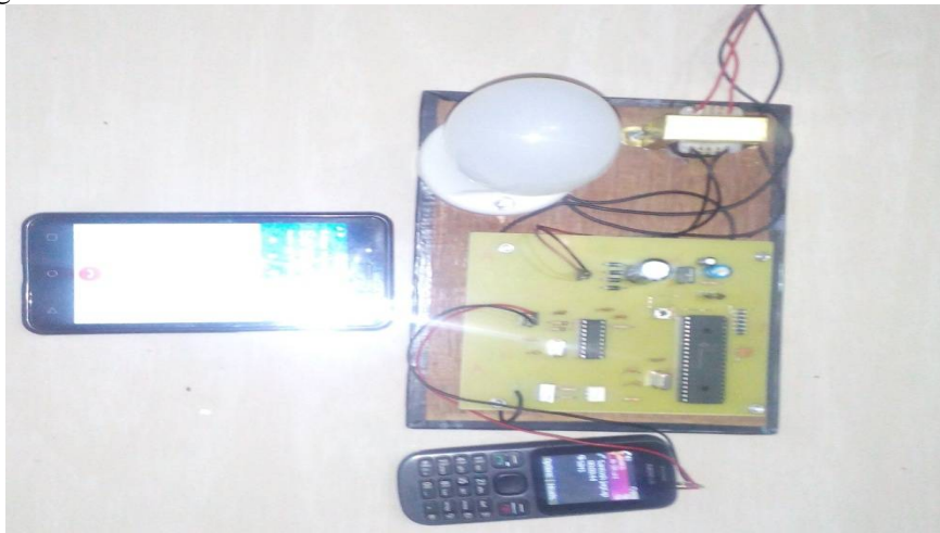
Fig.1. Initial condition Fig.1 This figure indicates the initial condition of controlling of ac lamp through mobile phone. when we call from another mobile phone ,the mobile phone at receiving side should be put on auto answer mode at that time initial condition of our project
