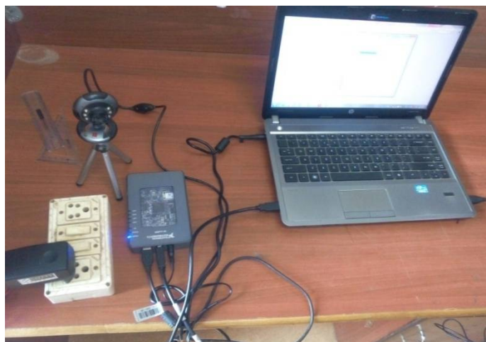
Figure(5): MyRIO Interfacing with camera
