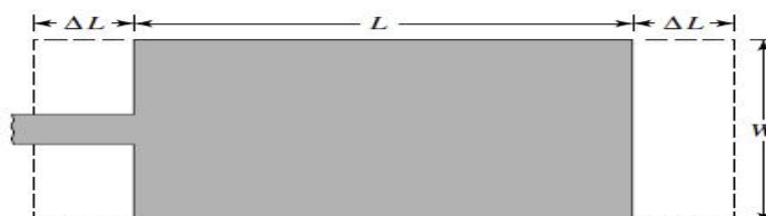
Fig 4. Physical and effective lengths of rectangular microstrip patch
