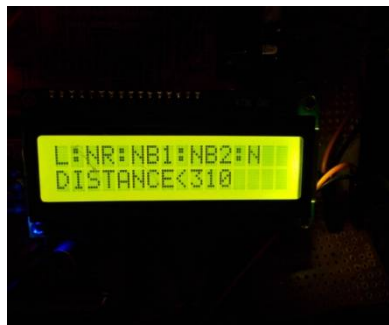
Fig 10: LCD display shows distance measured by the ultrasonic sensor
