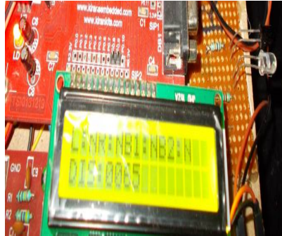
Fig 11: LCD display shows distance measured by the ultrasonic sensor is less than the reference distance.
