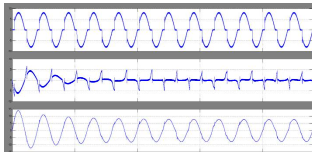
Figure.11. Load, Compensation & Source Current for \phi = 30^\circ
