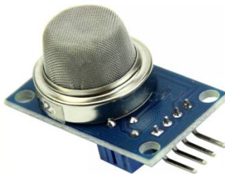
Fig. 4 GAS sensor (MQ-2)
