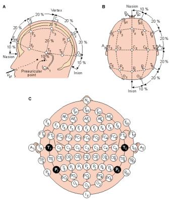
Fig. 1 The 10-20 international system seen from left (A) and above the head (B). The letters F, T, C, P and O stand for frontal, temporal, central, parietal, and occipital lobes. Even numbers identify electrodes on the right hemisphere, odd numbers those on the left hemisphere, and "z" (zero) refers to electrodes placed on the midline. (C) Location and nomenclature of the intermediate 10% electrodes, as standardized by the American Electroencephalographic Society [1].
