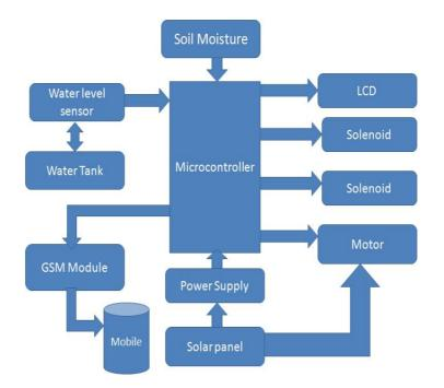
Fig. 1: Praposed block diagram
