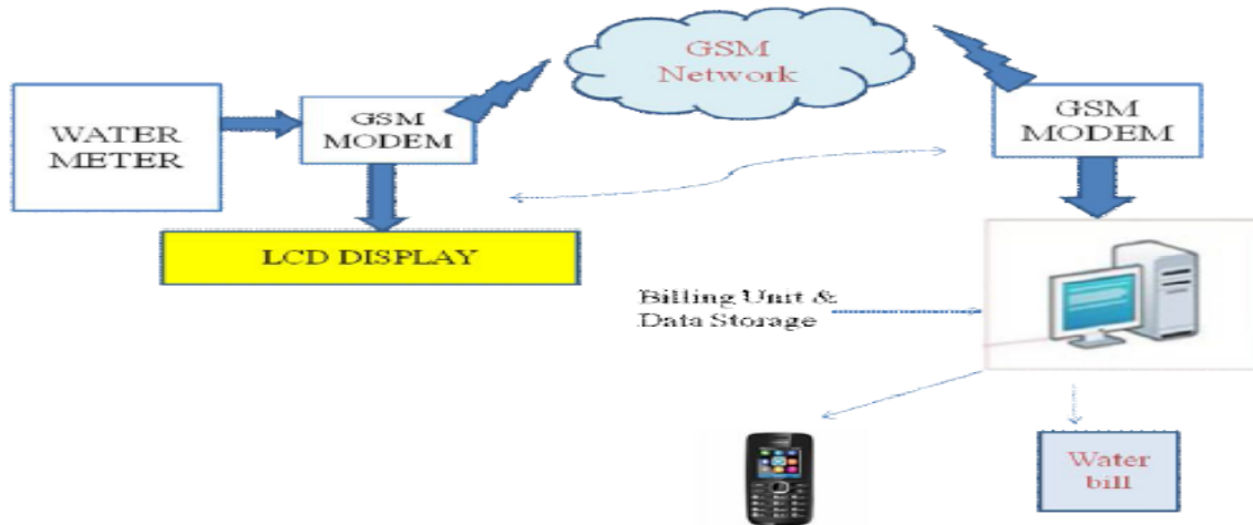
Fig. 1 Block diagram of GSM based automatic water meter reading system [1].
