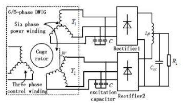
In the DWIG, two sets of stator windings are present, and an SEC is connected to the control winding, which results in increased complexity of the voltage buildup process when compared with a traditional IG. Considering that no-speed sensor exists in this system, the entire voltage buildup process is divided into three steps, namely, frequency search, generation in an open loop, and generation in a closed loop.
