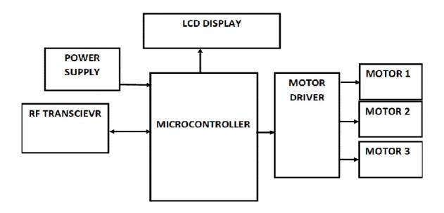
Fig. 3. SHELF END BLOCK DIAGRAM
