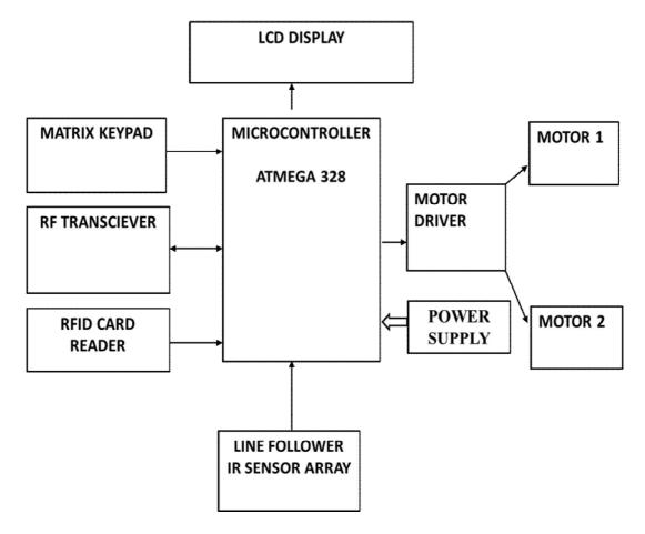
Fig. 2. ROBOT END BLOCK DIAGRAM
