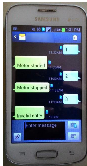
Figure 6 snapshot of user mobile phone protruding SMS interaction between user and SMS starter
