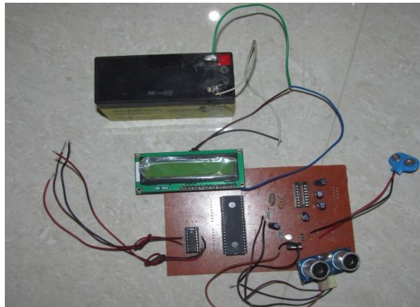
Fig. 3 Distance measurement using one ultrasonic sensor.
