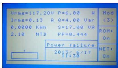
Figure 11: A typical utility power failure event on the MIU LCD display
