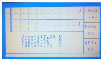
Figure 10: Harmonics measurement result by the proposed smart meter system in power quality monitoring mode
