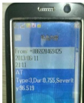
Figure 8: Typical alarm message sent to the user's cellular phone through GPRS mode
