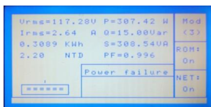
Figure 6: Typical test results for electric power parameters measurement by the proposed smart meter prototype for a power line in laboratory
