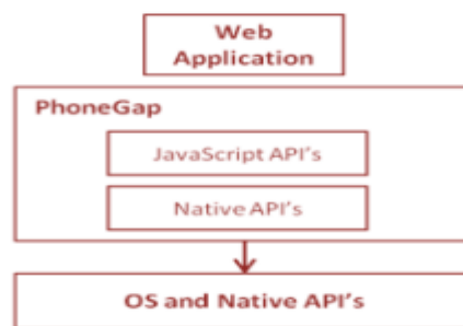
Figure 2: interfacing layers of the phonegap architecture
