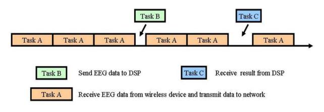
Fig..4. Time series diagram of multitask scheduling mechanism
