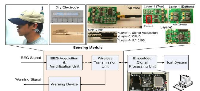
Fig1. Block diagram of the proposed BCI system.
