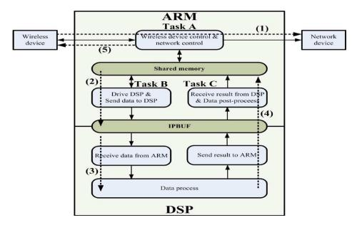
Fig.3. Software structure of the embedded system and the data processing flow.
