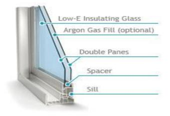
Figure 3:- Double glazed window (structure)
