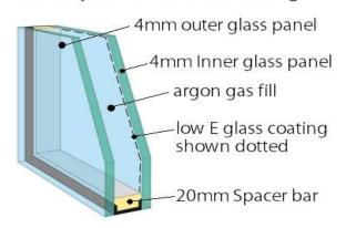
Figure 5:- Thermally efficient double glazed window
