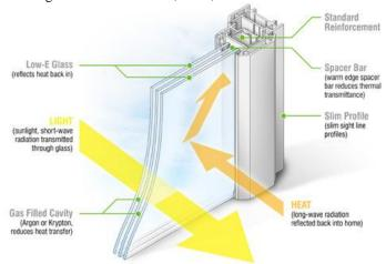
Figure 7:- Triple glazed window (working)
