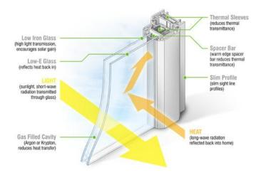
Figure 4:- Double glazed window (working)
