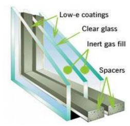
Figure 6:- Triple glazed window (structure)
